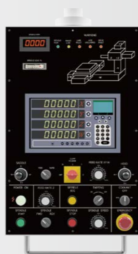
B version (For DRO brand: NEWALL & FAGOR) For the B version control panel, the W and Z axis will be reversed. Z = Spindle travel, W = Saddle travel
